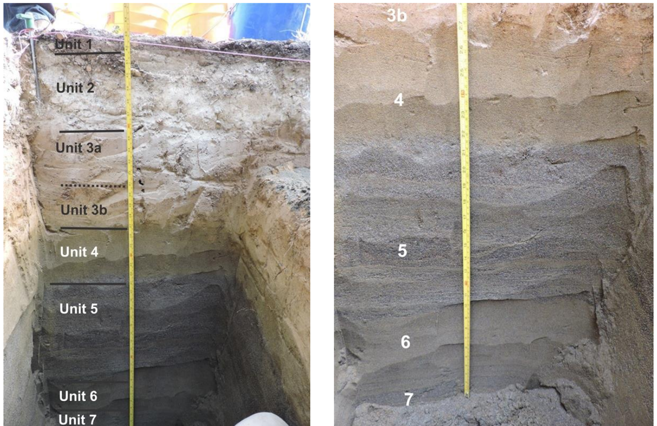
Figure 64. Sedimentary Strata, DML-09, July 20 – see table below for Unit descriptions
